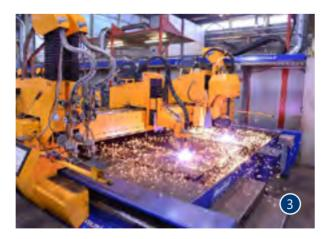
For the company Doppelmayr MicroStep installed a powerful drilling machine of the DRM series 11 and two plasma and oxyfuel cutting machines of the MG series with two gantries 2 + 3 each. The two MG machines are each equipped with a CCD camera 4 for maximum precision when cutting pre-drilled parts.
