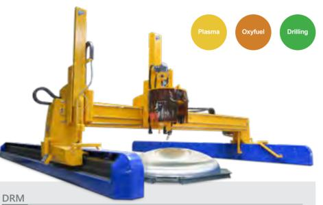
DRM is a heavy-duty CNC cutting machine designed for a wide range of dome, plate and pipe cutting applications. Its robust gantry allows a vibration-free operation of heavy equipment such as automatic oxyfuel triple torches or a 120° rotator with Z-axis stroke 1,500 mm for cutting of dished ends. DRM can be delivered also as a high-performance drilling machine with special drilling table.
