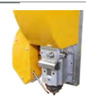
Laser tool station for fiber laser 2D
