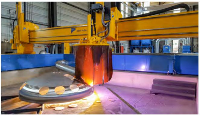
When designing the plasma cutting machine, the focus was on the precise and flexible processing of domes. A special dome cutting table supports domes from 500 mm up to 5,500
