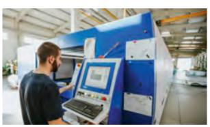
Faddikorr opted for two CNC cutting machines from MicroStep: fiber laser machine MSF with a straight tool station, with work area 6,000 x 2,000 mm (below), and a sturdy 3D plasma cutter DRM equipped with a pantographic plasma rotator capable of tilting up to 120° designed solely for cut-
