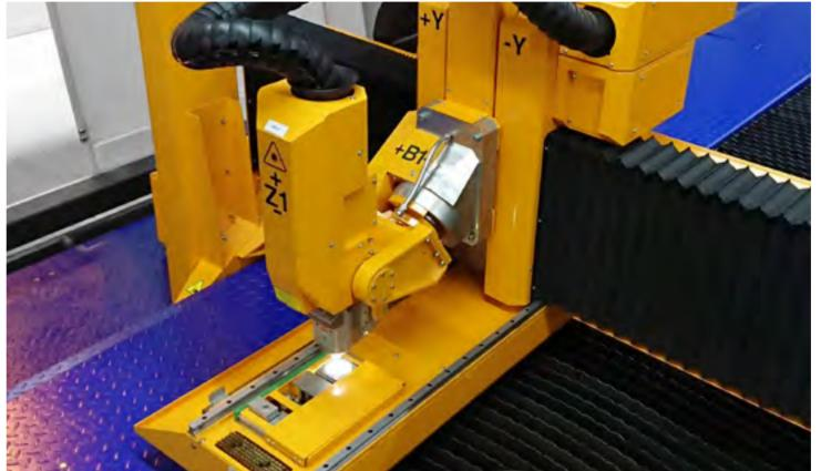
Above: Chantiers de l'Atlantique opted to invest into a large-scale fiber laser cutter MSF Max. It is a 50 m long machine with two 21,000 x 3,500 mm cutting zones.
