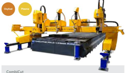
This robust, high-precision CNC machine is designed especially for multiple-shift high-performance plasma and oxyfuel cutting. It allows cutting of steel up to 300 mm thick, bevel cutting with a pair of oxyfuel triple torches or rotators, parallel cutting with up to 8 torches, drilling up to Ø 40 mm, inkjet, micro-percussion or laser marking, as well as pipe and dome processing.
