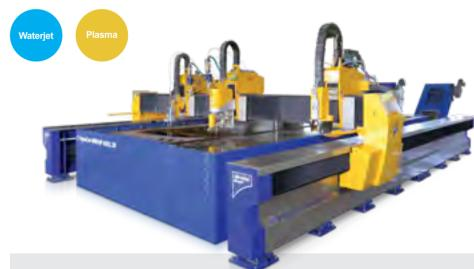
AquaCut is a versatile waterjet cutting machine designed for processing of a wide variety of materials including those that cannot be subject to thermal or mechanical stresses. The machine can be equipped with a 5-axis waterjet rotator, as well as combined with plasma cutting, pipe and profile cutting or tapping. Further features include ABP technology and taper compensation (ABC).
