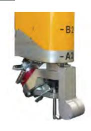
5-axis rotary bevel head for waterjet enables bevel cutting of all types of materials up to 45°. Adaptive taper compensation (ABC) and periodic height sensing (PHS) are included by default.
