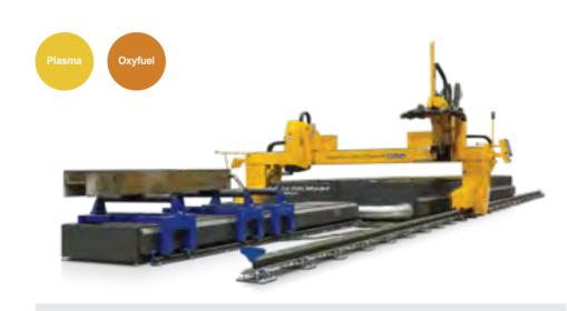
ProfileCut is a machine dedicated for production of steel structures. Besides optional pipe and plate cutting zones, ProfileCut's main cutting area is dedicated to processing of structural beams such as I, H, U or L. To enable precise division as well as cut-outs in required spots on the beam, the machine is equipped with a laser scanner for measuring of the true shapes of beams.
