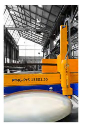
Maximum precision in dome cutting is made possible by MicroStep's mScan technology. In the process, a laser scanner integrated into the portal determines the 3D surface geometry of the workpiece in advance.
