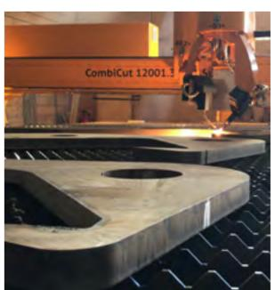
For the jobs at Solintal (e.g. 45° Y-bevels on parts 160 mm thick) oxyfuel was naturally the technology of choice. The movement capabilities of rotator allow to cut a great variety of contour shapes. A high output accuracy is ensured by the possibility of auto-calibration of the oxyfuel rotator – thanks to MicroStep's patented ACTG® technology.
