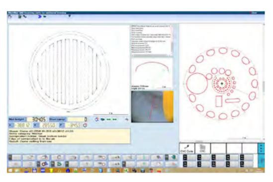
Thanks to the mScan technology, the 3D scan of a dome enables to determine production-related deviations from the ideal contour that then could be compensated for accordingly during cutting.
