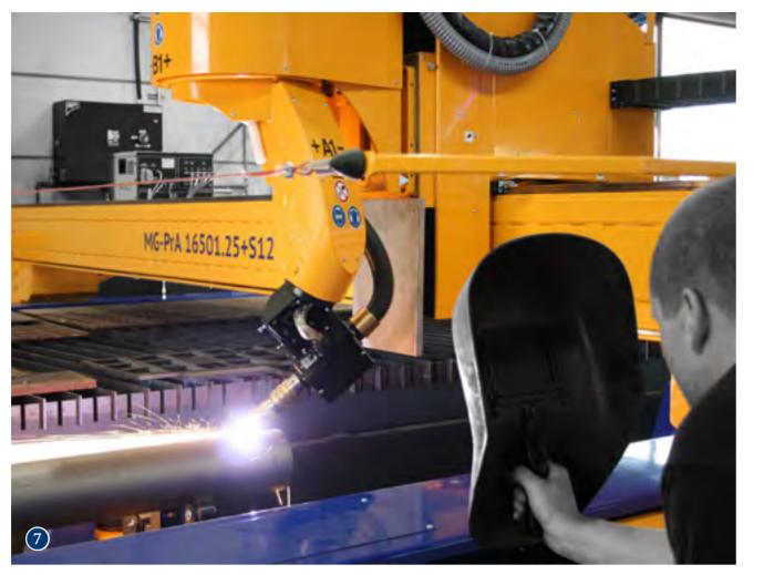
MicroStep machines provide two types of beveling
