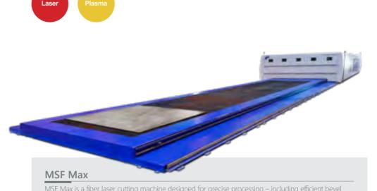
MSF Max is a fiber laser cutting machine designed for precise processing – including efficient bevel cutting – of large-sized components. The machine offers an extensive production versatility, including 2D cutting, bevel cutting up to  $45^{\circ}$ , drilling up to  $\emptyset$  30 mm, tapping up to M20, countersinking and marking.
