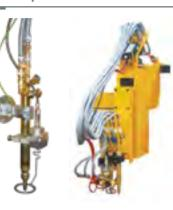
Oxyfuel tool station with manual tilting possibility up to ±45°. Fully automatic gas console with preset parameters ensures stable quality of cuts and best efficiency. Multi-tool version enables stripe cutting with stripe width  $\geq$  70 mm.
