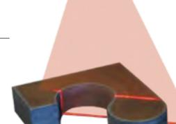
Laser scanner dedicated for scanning of both the contour and position of a straight pre-cut part in ABP feature – additional cutting of bevels for weld edge preparation. ABP technology is available for plasma, laser, oxyfuel and waterjet cutting
