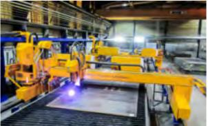
The combined plasma and oxyfuel cutting solution at MAP Prinzing Brennschneidtechnik GmbH enables bevel cutting with plasma, 2D oxyfuel cutting, drilling, tapping and marking on two gantries. At the request of the company, a tool magazine for 16 tools was added.
