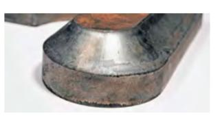
Close-up view of a cut part with added bevels.
