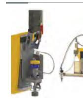
Waterjet tool station for cutting of all types of materials. Multi-tool version can carry up to 4 water jets on a single Z lifter.
