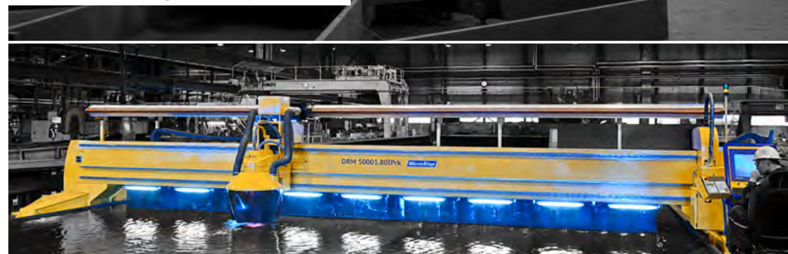
DRM machine with work area 50 x 8 meters and a water table for underwater plasma cutting
