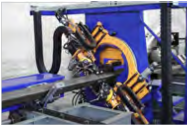
DS-B: Automated drilling and marking of hollow profiles
