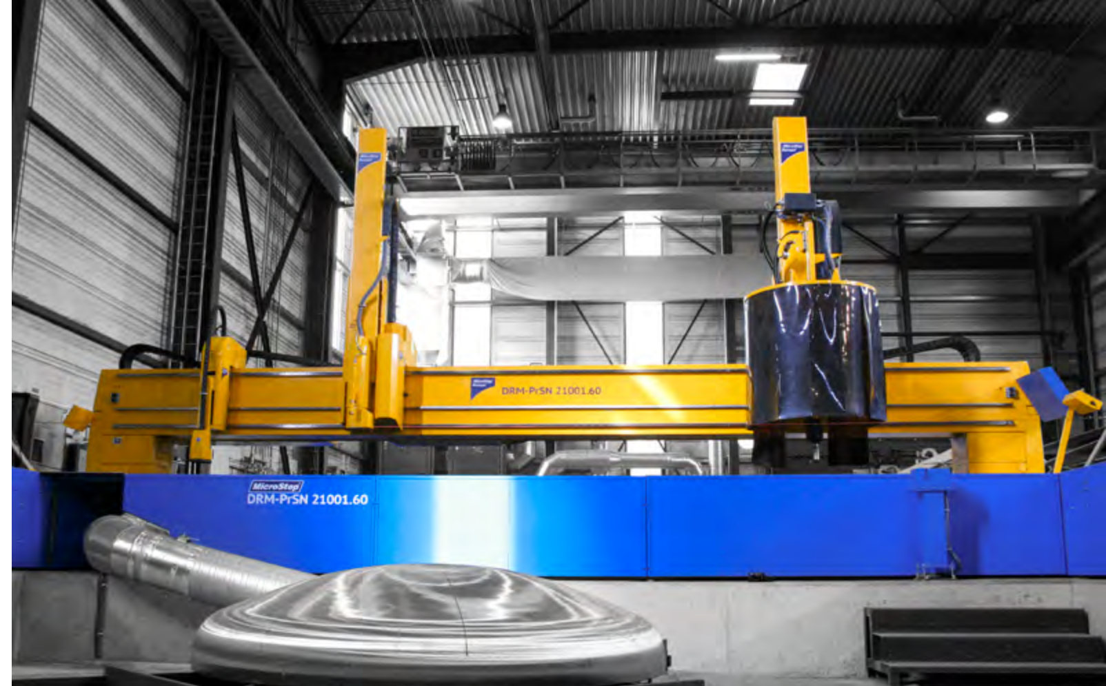
DRM machine for cutting of tank ends up to Ø 5,500 mm
