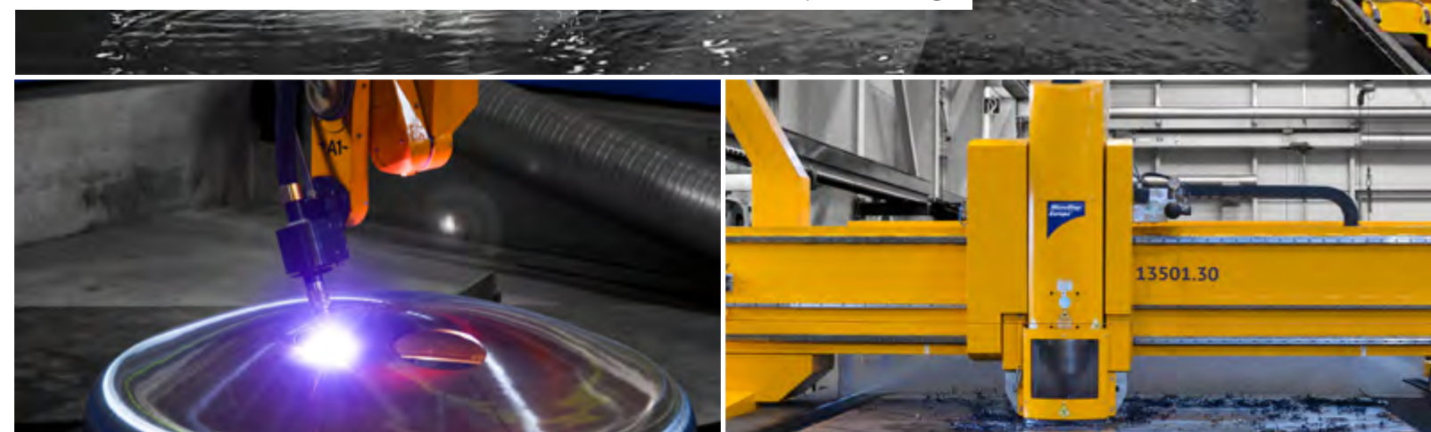
Tank end processing on DRM, with a 3D rotator with tilt angle up to 120°
