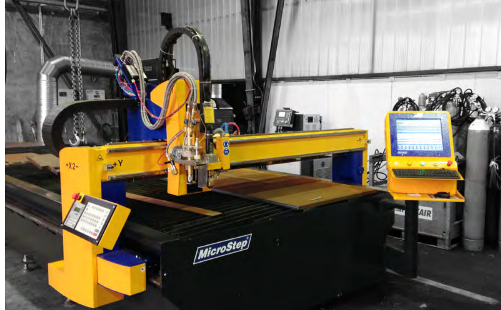
MasterCut Compact machine designed for small and medium-sized businesses
